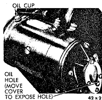
Figure 6—Lubricating Generator (1942 Models, Typical of 1936-41 Models)
