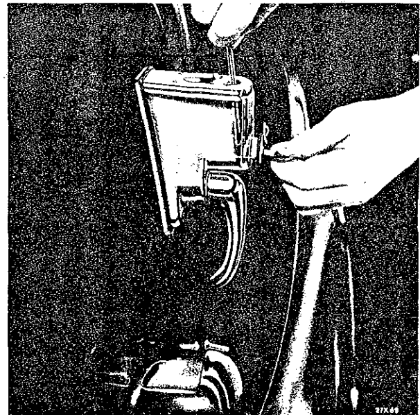
Figure 5—Depressing Plunger to Remove Luggage Compartment Lock Cylinder (1942 Model, Typical of 1940-41 Models)
